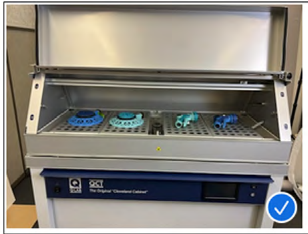
Figure 2. QCT tester with humidity enclosure attachment illustrating enclosed condensation
