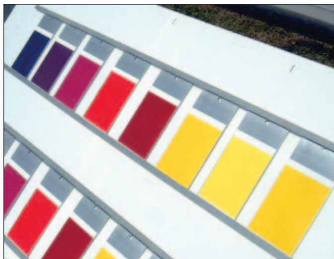
GATF technical staff selected eight representative lithographic ink colors printed on a standard substrate for fade resistance testing.
