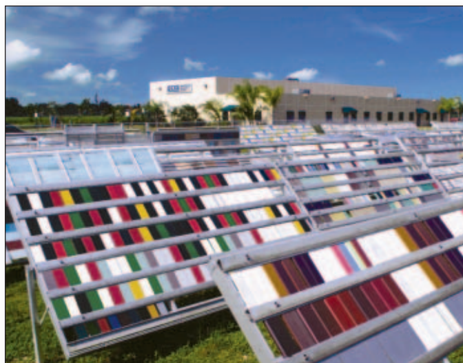
Q-Lab Weathering Research Service Test Facilities in Florida and Arizona performed fade resistance testing of lithographic inks in extreme environments.
