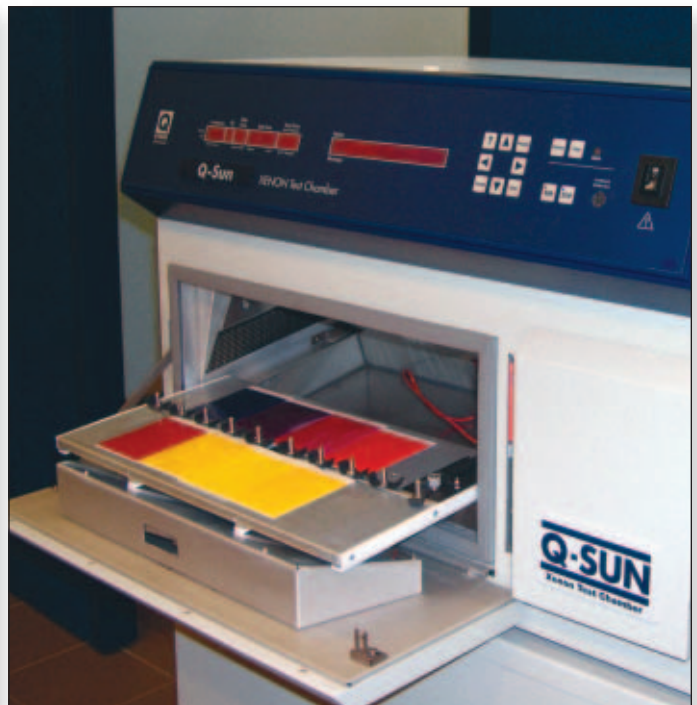
An ideal test program includes natural outdoor exposures in Florida or Arizona benchmark locations and accelerated lab testing in a Q-Sun Xenon Test Chamber.
