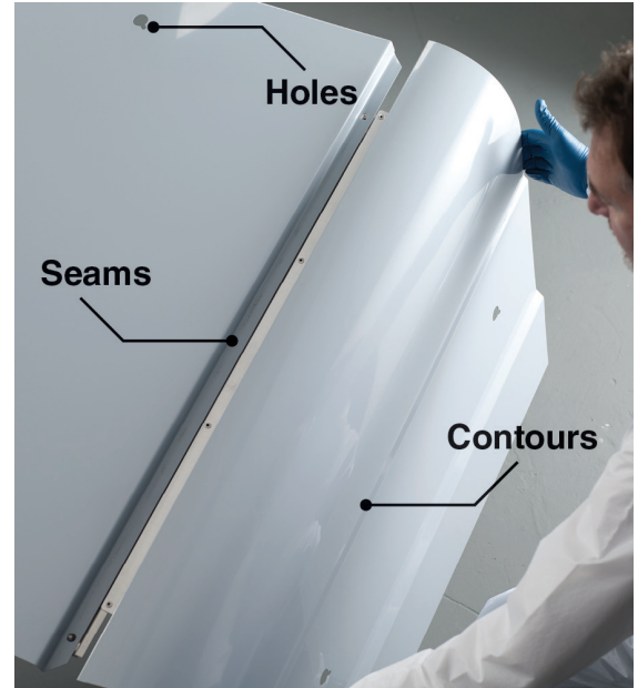
Seams, holes and contours provide an accurate representation of real automotive hoods and fenders.
