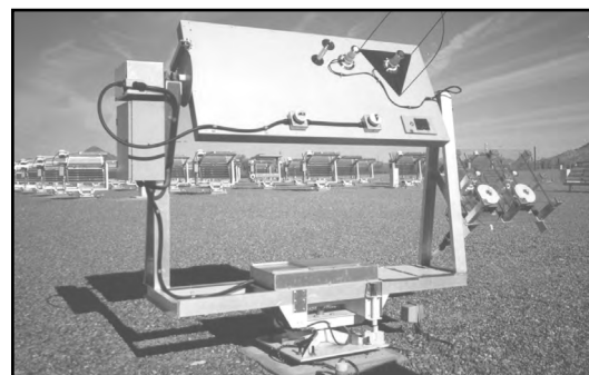
Figure 11 - Radiant dosage calculations are made from data collected from a solar tracking device equipped with two Eppley TUVRs and a Normal Incidence Pyrheliometer.
