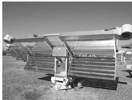
The dual Q-TRAC unit has twice the capacity of the original Q-TRAC system design.
