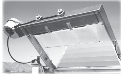
Figure 7 - Four spray nozzles apply a fine spray of highly purified water onto the specimens at a rate of 0.20-0.25 GPM.
