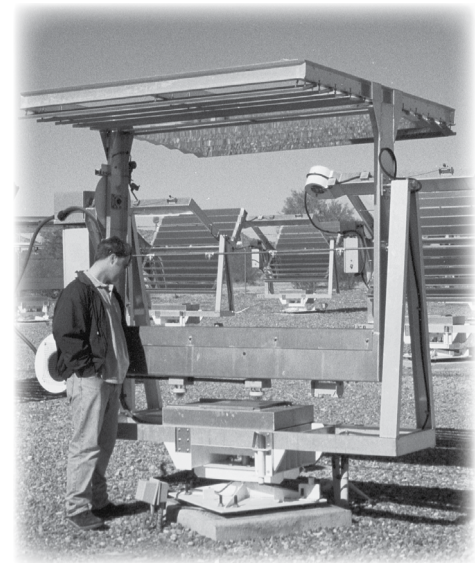
Figure 8 - The 5 degree inverted lock-down position simulates dew formation on specimens during nighttime wetting. The lock-down position also allows easy specimen mounting and evaluation.
