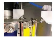
Dual spray is available for the Xe-3 only. It allows a second liquid solution, such as an acid rain or soap solution, to be sprayed onto test specimens. The system consists of a large external reservoir, centrifugal pump, and a filter.
