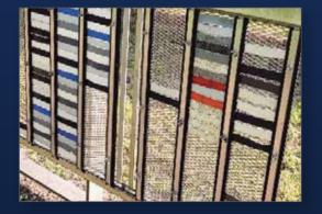
Located near Miami, Q-Lab Florida's outdoor testing site is ideal for repeatable and realistic outdoor exposure testing for products in both temperate and tropical regions.
