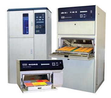
A variety of Q-SUN models offer all the flexibility and features you need in a xenon arc tester. Three dimensional products are easily accommodated on the flat specimen tray of both Q-SUN Xe-1 and Xe-3 xenon chambers. The Q-SUN B02 chamber is specifically designed with a rotating rack for ISO 105 B02 textile lightfastness testing.
