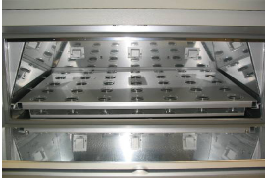
Figure 3 - Water collection set-up in a flat array accelerated weathering device.
