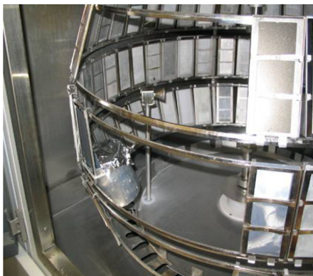
Figure 2 - Collection of water dripping off of standard paint panel during accelerated weathering in a rotating drum device.
