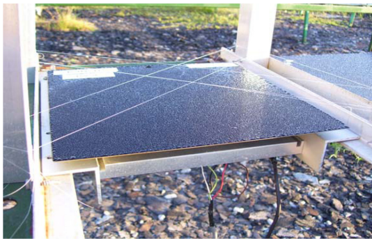
Figure 6 - Paint panel attached to load cell for water exposure study. Load cell is underneath horizontal paint panel.
