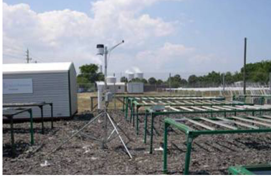
Figure 5 - Test site where FL water exposure was measured. Note weather station next to panel racks.
