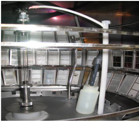
Figure 1 - Experimental set-up for collecting water from spray nozzles during testing in a rotating drum accelerated weathering device.
