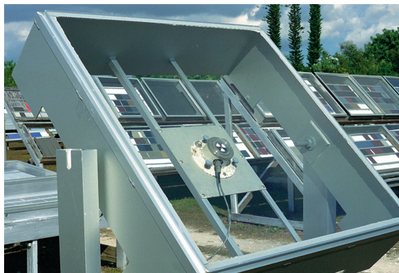
Figure 2 - Total Hemispherical Pyranometers can measure total sunlight energy directly and under glass.
