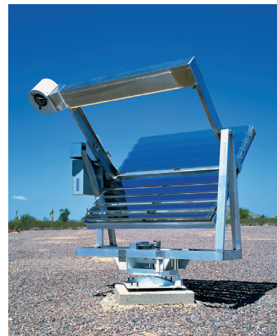
Figure 5 - For a detailed description of this energy calculation method, see ASTM G90, Standard Practice for Performing Accelerated Outdoor Weathering of Nonmetallic Materials using Concentrated Natural Sunlight. G90 is available from the American Society for Testing and Materials, 100 Barr Harbor Dr., W. Conshohocken, PA 19426
