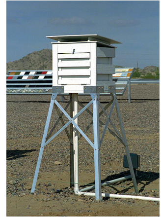
Figure 9 - The World Meteorological Organization standard Instrument Shelter houses temperature and humidity devices. It is designed to protect instruments, yet allow accurate sensing of ambient air conditions. The slotted sides allow free air circulation.
