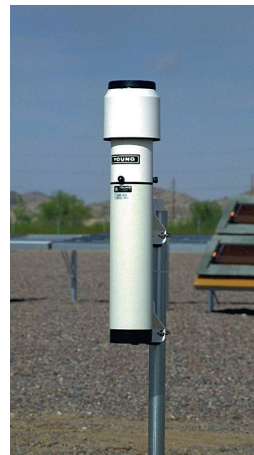
Figure 8 - The Rain Gauge measures the amount and duration of rainfall, along with the rate of accumulation.
