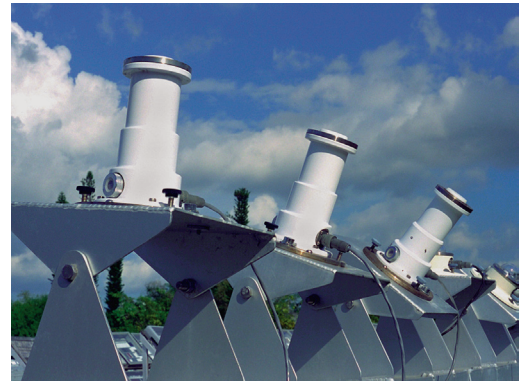
Figure 1 - Total Ultraviolet Radiometers (TUVRs) are mounted at the common exposure angles (e.g. 45° South, 5° South, Latitude Angle) to measure UV radiation from the sun.
