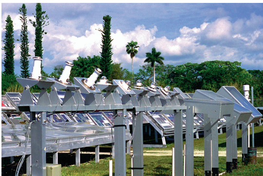
Figure 6 - Miami, Florida Installation. Climate measurements are taken in the specimen exposure area to reflect the actual test conditions. (Miami, Florida: Subtropical); (Phoenix, Arizona: Desert)
