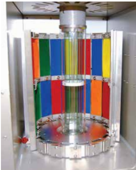
Specimen mounting and evaluations are simplified with specially-designed specimen holders in the Q-SUN Xe-2 model.
