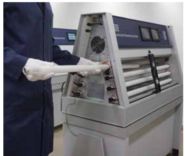
Irradiance-controlled QUV models do not require lamp rotation. However, when the time comes to change a lamp, double sided access makes the job easy to perform.
