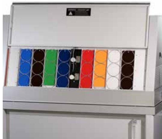
A QUV tester can accommodate 48 specimens.
