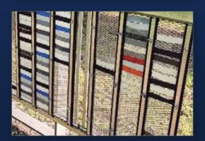
Located near Miami, Q-Lab Florida's outdoor testing site is ideal for repeatable and realistic outdoor exposure testing for products in both temperate and tropical regions.
