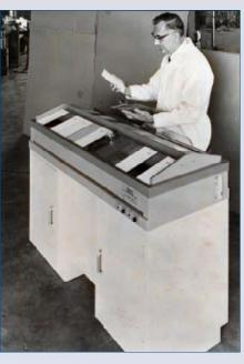
**1965** QCT "Cleveland Condensation Tester" introduced by Q-Lab. This precursor to the QUV provides condensation only, but no UV.
