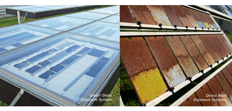
Direct Exposures are intended for materials and products that are expected to experience the full effects of weathering - sunlight, heat, & moisture. Common materials include coatings, plastics, and any finished product intended for outdoor use.
