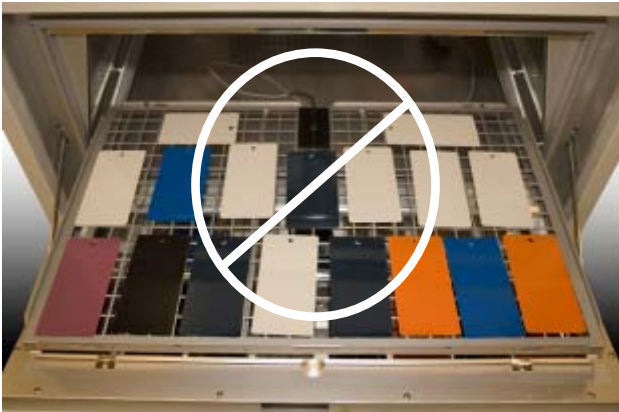
Figure 9.3g: Gaps between specimens on the open back tray affect cooling air flow.
