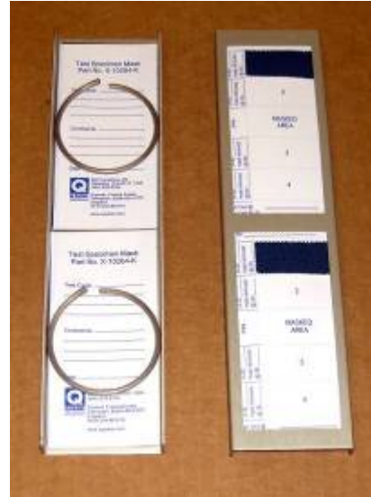
Figure 9.3t: Textile mask mounted in panel holder with one section of the mask removed.
