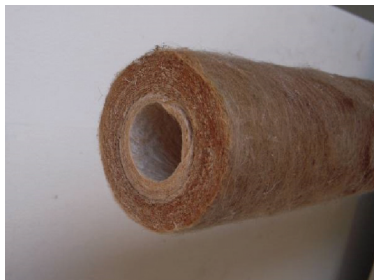
Microporous depth filter after one month of use at Q-Lab Arizona.
