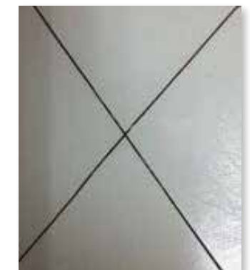
Paint applied to aluminum with pre-treatment B shows excellent adhesion performance
