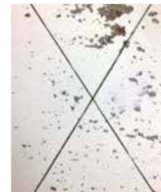
Paint applied to aluminum with pre-treatment A shows minimal adhesion failures
