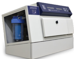
Specimens immersed in temperature controlled water during light or dark conditions rest on mesh insert.
