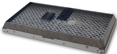
Specimens immersed in temperature controlled water during light or dark conditions rest on mesh insert.
