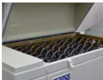
Figure 3 Large, heavy metal springs are mounted using the Rack-Level Grates.
