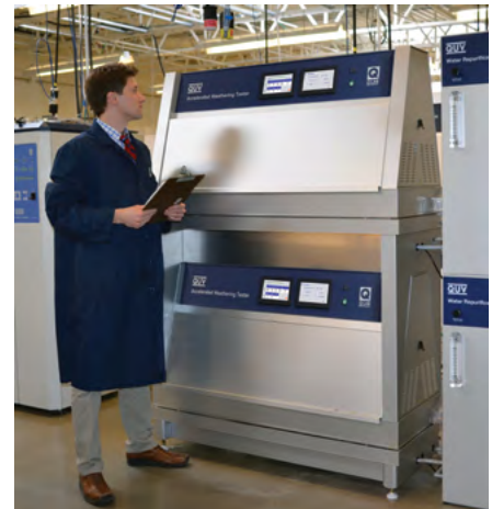
Stacking testers on the space saver frame allows easy access to both machines.
