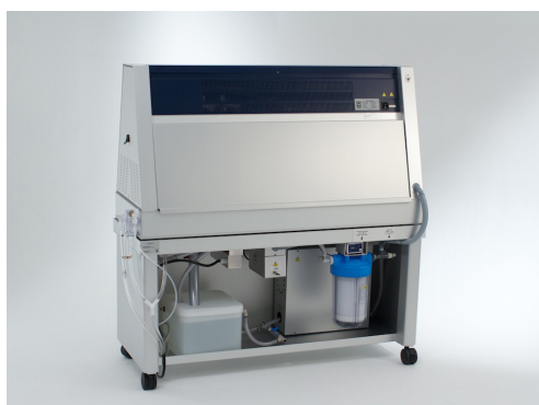
On new QUV test chambers, the water repurification system is integrated directly into the tester.
