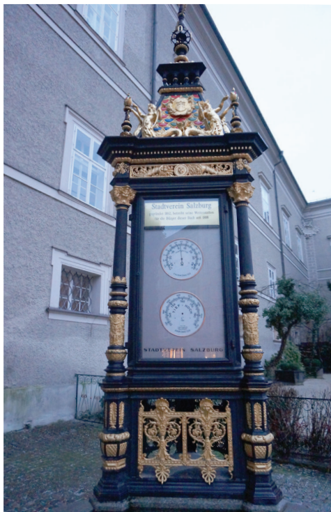
This late 19th century weather station in Salzburg, Austria was declared an historical landmark in 2007. Pictured is the side displaying the relative humidity. Hygrometers of this era commonly used human hair under tension, since it changes length depending on the moisture content of the air.
