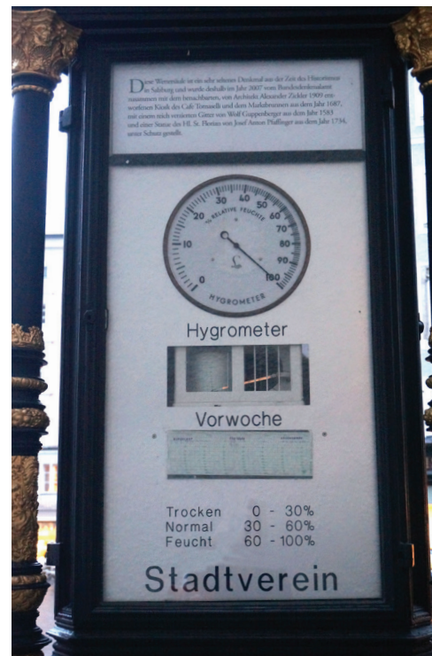
This late 19th century weather station in Salzburg, Austria was declared an historical landmark in 2007. Pictured is the side displaying the relative humidity. Hygrometers of this era commonly used human hair under tension, since it changes length depending on the moisture content of the air.
