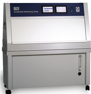
Figure 1 - QUV fluorescent ultraviolet-condensation apparatus
