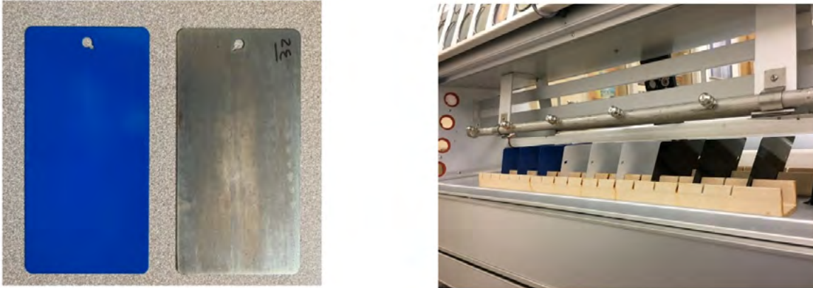
Figure 4. Painted and unpainted specimens (left panel) and specimens mounted in a QUV with painted side facing down (right panel).
